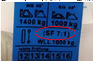
Slings are colour coded, but that does not mean a missing label is okay. If the label is missing, take the sling out of service. From there, visually inspect the sling for damage to the cover, end fittings, stitching, or significant colour change from UV. Finally, feel the sling for lumps or thinning areas with the outer cover.
