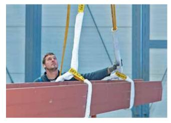
The white protective sleave on the sling provides edge protection. Edge protection is not only used against abrasion, but also increases the corner radius of the load putting pressure on the sling.
