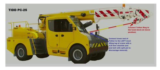
Please note: this tether must be kept clean and in good order at all times. It is strongly suggested that the tether be fitted as per the instructions with a bow shackle with the nut and bolt and split pin are used to discourage removal of the tether so that it is always there when travelling through a tunnel. This tether has been developed to allow the boom to be elevated no more than a maximum of approx' 5 degrees.
