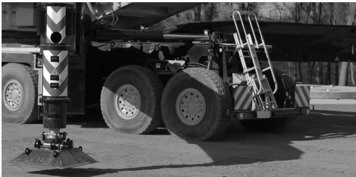
Example 7 - Outriggers extended and corresponding road width requirement
