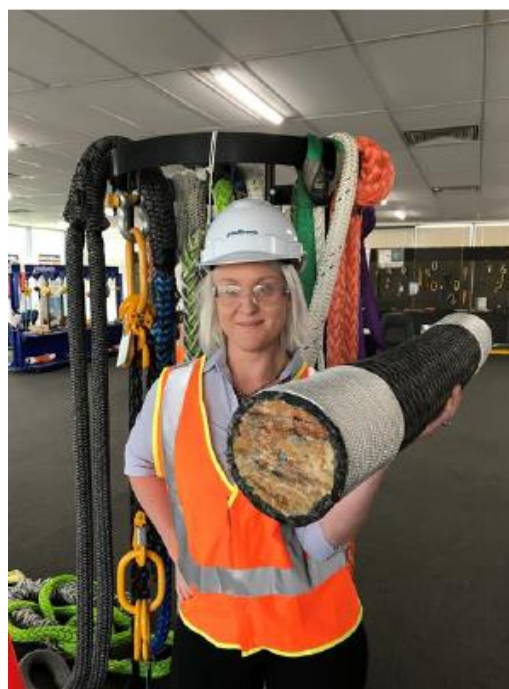
In the picture above, 138mm synthetic rope per meter mass is 10kgs versus steel core wire rope at 65kgs. Breaking strain -1440 tonnes versus 1155 tonnes.
