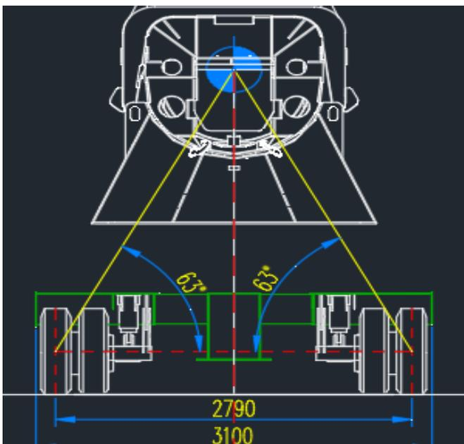
The other main factor at play here is the lateral force acting on the 20t boom as the float travels around a corner. This Centrifugal force is defined by the equation:
