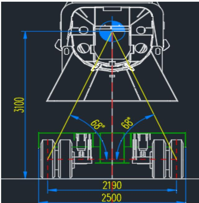
Crane booms can weigh up to 20t and the COG is 3.1 meters above the road. The triangle of stability is drawn off the centreline of the outside tyre in this case and I'm ignoring tyre deflection. In theory the stationary float will tip at around 19deg of tilt. If the float is widened to 3.1m then the stationary angle required to tip the float is much larger at 27deg. (I'm ignoring the float mass for simplicity)
