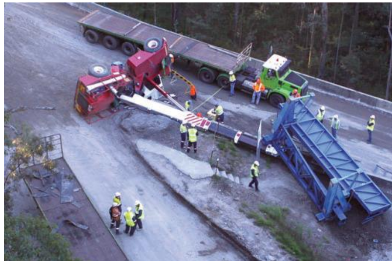
Figure 1: Articulated Crane Rollover when Carrying a Load [1]
